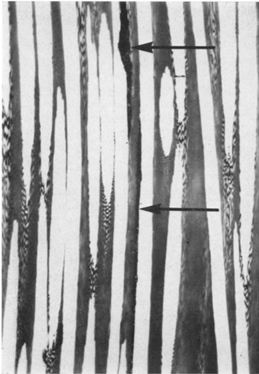
Figure 5 Microstructure of a longitudinal cross-section of a carbon-epoxy composite deformed at atmospheric pressure, showing evidence of longitudinal fracturing (cf. Fig. 1a). Compression axis vertical, \times 500 .
